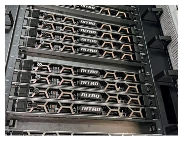
The core storage infrastructure integrates Dell-EMC PowerScale for scalable storage, while Karthavya QuickEdge Automation and Nitro servers form the backbone of the playout facility. Nearly 100 video servers manage up to 800 video ports, supporting the smooth operation of 500 channels.
